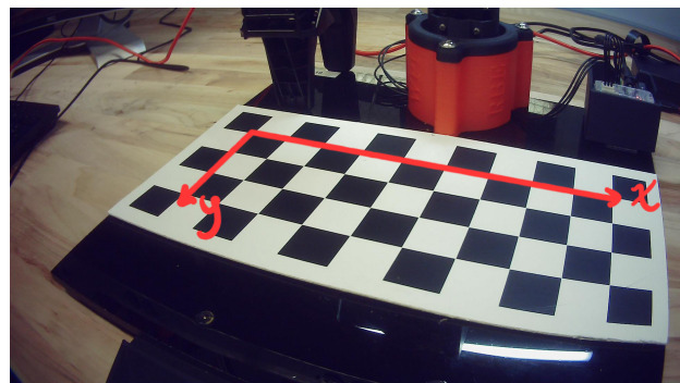
Fig. 5. Designated frame orientation for the checkerboard frame. Images with a different frame orientation were rejected from calibration of the camera
